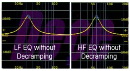
Normal digital EQs can sound harsh as the high and low ends are effectively squashed during EQ'ing. The Trakker tackles this by the use of decramping.
