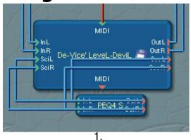
Connect an equaliser between the sidechain inputs and outputs of the LeveL-DeviL as above. (NOTE:the sidechain outs on the leveL-DeviL are 'post' (after) the detection circuit. This gives a very different response than just connecting the InL + InR to the SciL + SciR as with standard compressor designs. This is a special feature of the LeveL-DeviL)
