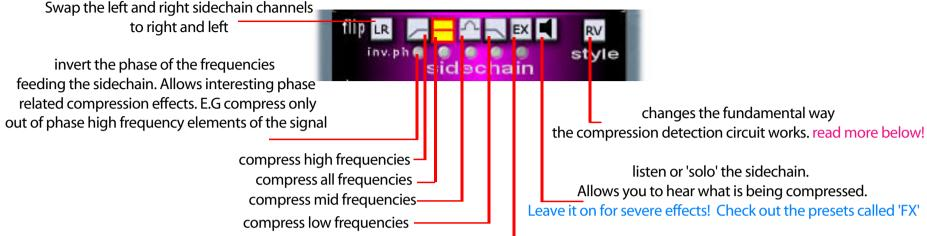
engage external sidechain circuit. Usually an EQ patched between the SCo (L+R) channels and the SCin channels of the sLiM-JiM module in the Scope 'Project window'. Doing this allows you to control exactly which frequencies you want to compress. You could insert absolutely any effect into the sidechain for some very strange compression effects. Have a play!
