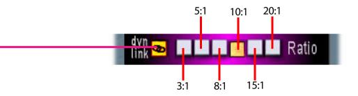
here you can adjust by how much the signal is reduced as the compressor kicks in. With all switches off, the compressor goes into limit mode (>30:1 ratio).
